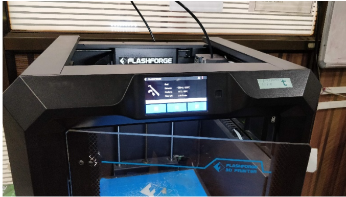
Our pen being 3D-printed using the Flashforge Gider II. It took around 2 hours 13 minutes to print. 12 grams of ABS plastic was required for the entire assembly.
