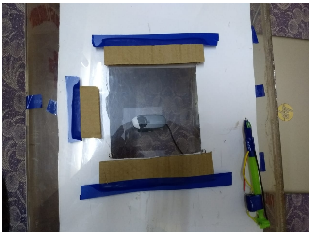
The plastic cuboidal enclosure has a webcam placed on the bottom surface. Three cardboard slits at the top ensure that the paper does not shake while the user is writing. White chart-paper is used to prevent light composed of unwanted colours from reaching the webcam.
